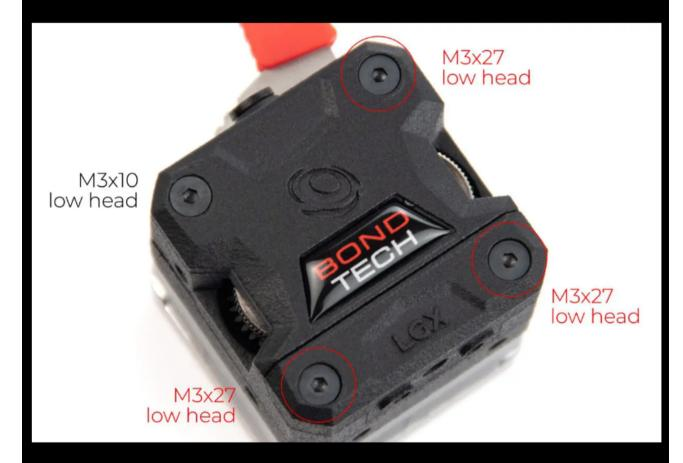
To use a plate in between the stepper motor and the extruder, you need to replace the stock M3x27 low head screws with the 3 M3x30 low head screws we send in the accessories bag, which are compatible with printer plates of thicknesses between 0.3 and 2.6mm.
