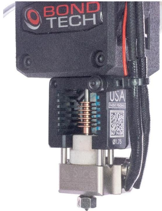
*Figure 14. Mosquito™ with temperature sensor, heater cartridge, fan, and nozzle installed with strain relief on the Bondtech BMG-M*
