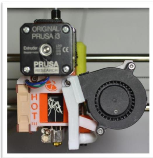
Figure 9. Mosquito installed on a Prusa printer with the Noctua fan that comes with the Prusa
