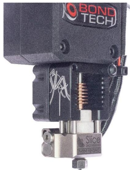
Figure 5. Mosquito™ mounted to the Bondtech BMG-M
