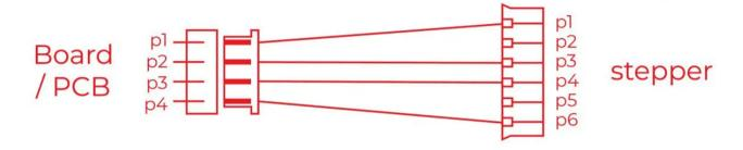
After the start of service, if the **LGX**® is turning in the wrong direction, swap the top (or bottom) pair of wires to make a correction:
