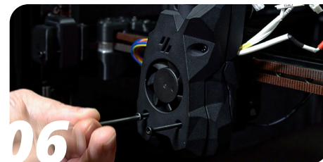
06 Add your screws for the front, make sure the upper ones are M3x16 SHCS if you're using the LGX lite
