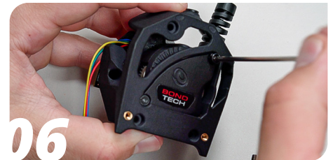
06 Change the two front screws on the extruder one at a time, replace them with M3x30 SHCS
