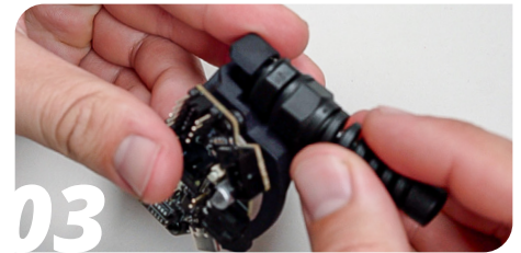
03 Remove the lower nut from the PG7 and screw it into the mount
