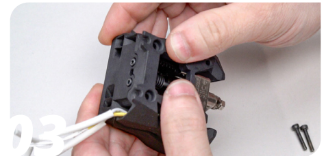
03 Place the hotend mount rear piece on the assembly
