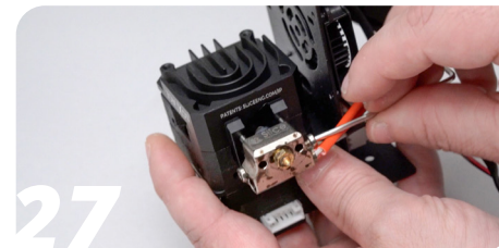
27 Add the heater and thermistor retention screw and tighten with a 2 mm hex key.
