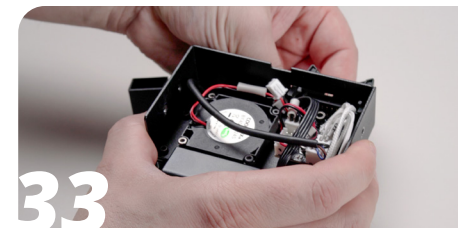
33 Route the wire from the 5015 from the front to the back and connect it to the board.
