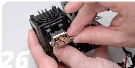
26 Add the heater and thermistor to the hotend.
