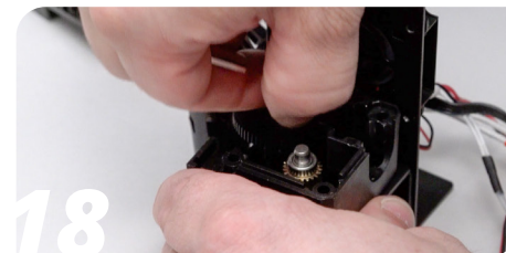
Remove the main extruder gear.
