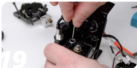
Undo the screw in the center of the main extruder gear bearing.
