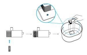
3. Insert the water pump's USB cable through the hole at the back of the water tank, starting from the inside and extending outward.
