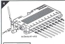
Crimp the DC positive wire (+) with the included round terminal. Pass the wire through the included insulator and connect to the screw terminals. Cover the terminals with the insulator properly. Crimp the DC negative wire (-) with the insulated 0.250" female terminal and insert into the negative quick terminal on Control Box.
