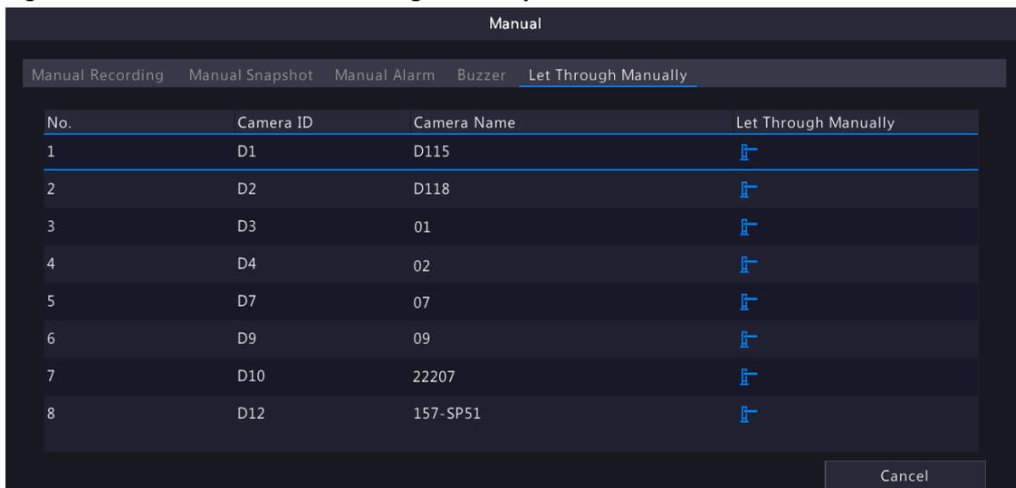
2. Click the corresponding
