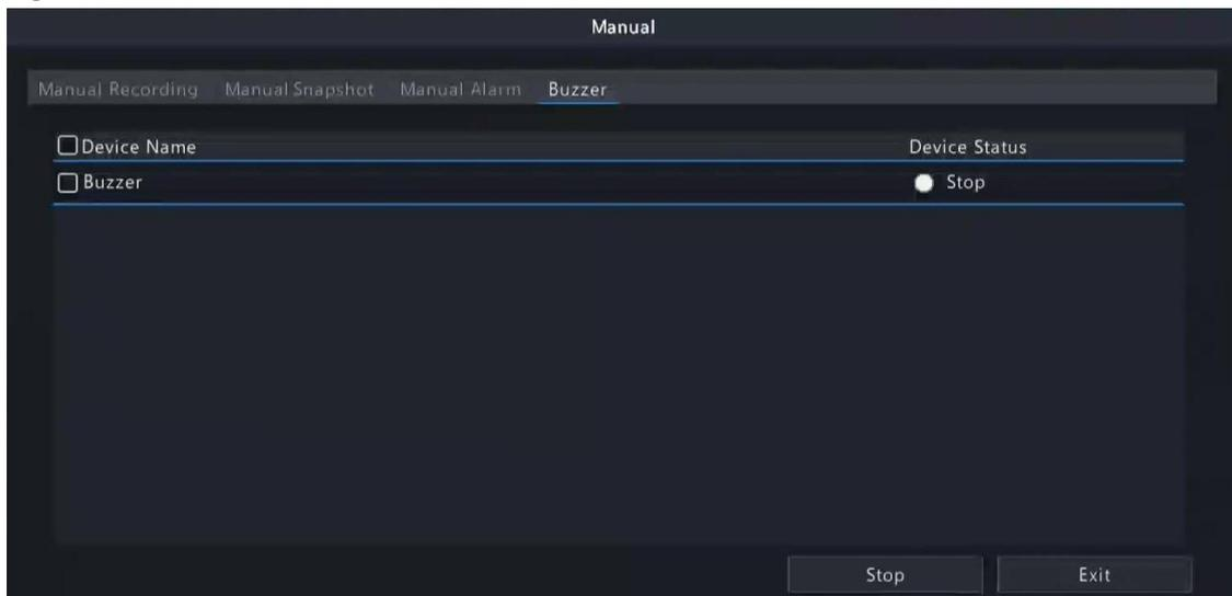
2. To stop the buzzer, select the buzzer (in Started status) and then click **Stop**.
