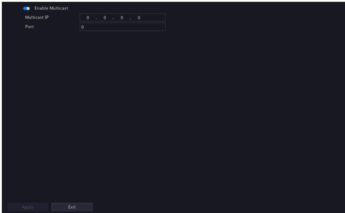
2. Enable multicast, enter the multicast IP address, and port number.
