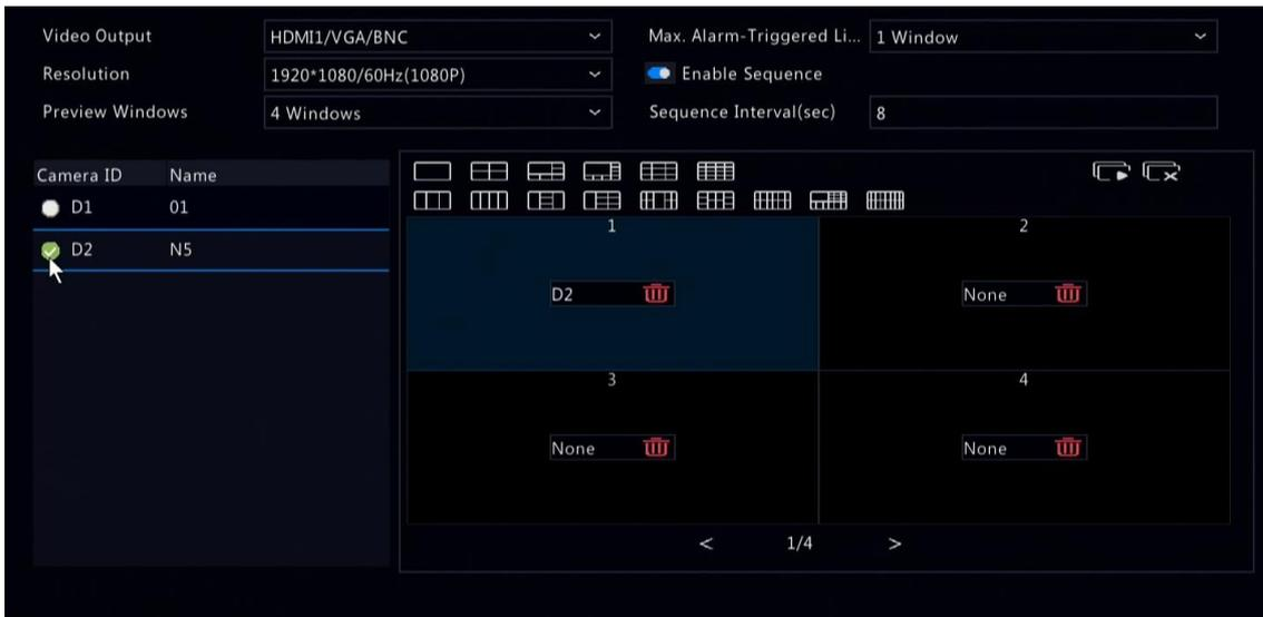
**Note:** On the left-side channel list,
