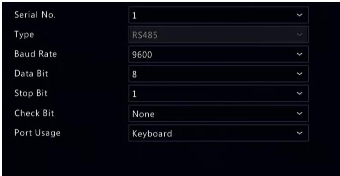
The screenshot shows a configuration interface for the Serial Port. It consists of seven rows, each with a label on the left and a dropdown menu on the right. The settings are as follows:
