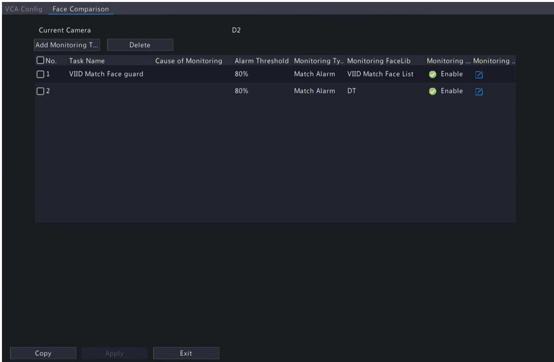
4. Configure monitoring tasks. A monitoring task of "DefaultList 80% Match Alarm" is enabled by default. You can click to modify it or click **Add Monitoring Task** to add more.
