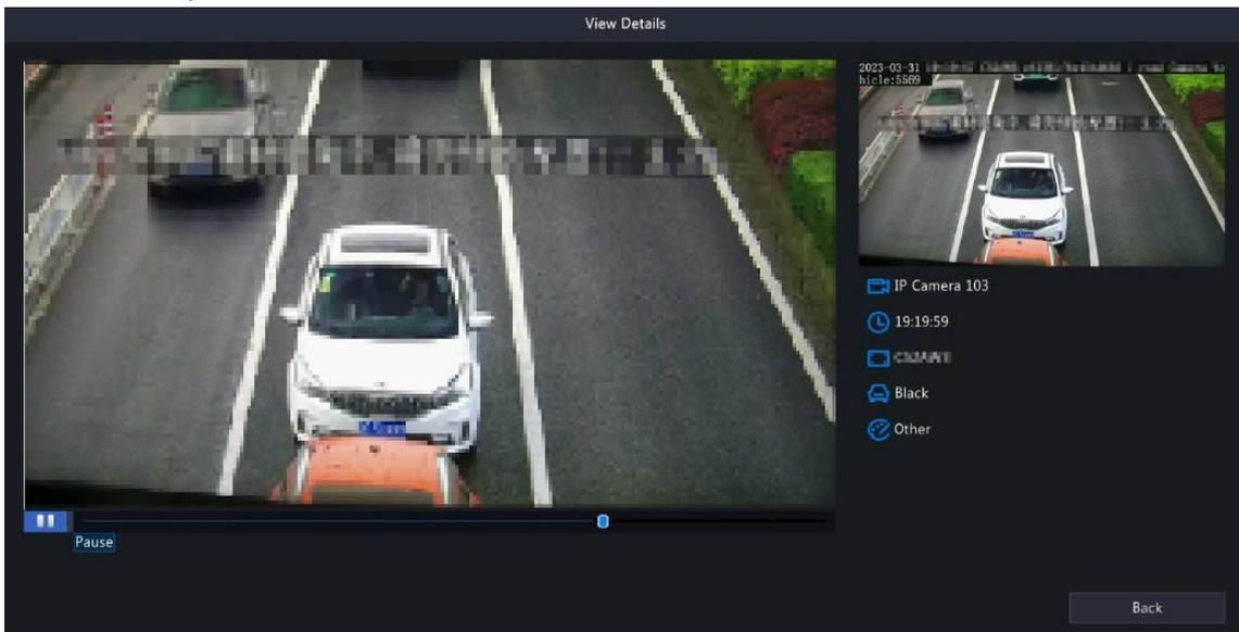
In the **View Details** dialog box, a 10s video (5s before and 5s after the snapshot) is automatically played on the left, and the snapshot and its detailed information including camera name, time, license plate number, vehicle color, and plate color are displayed on the right.
