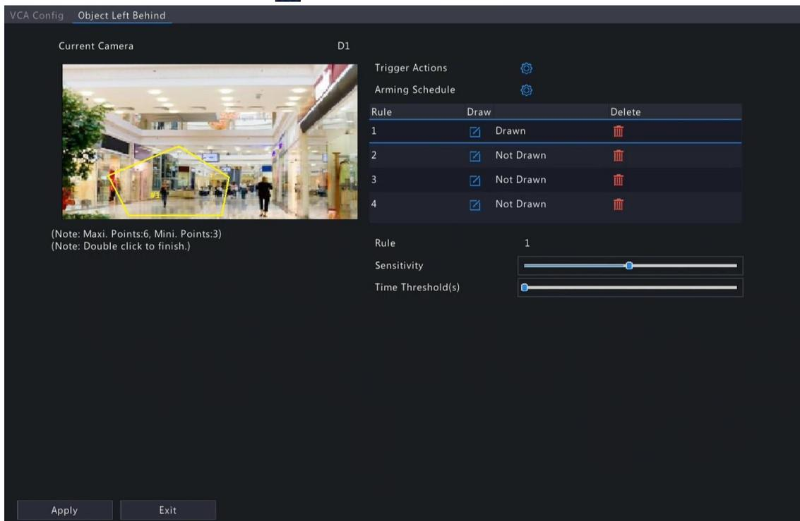
The screenshot shows the 'VCA Config - Object Left Behind' interface. On the left, a camera view labeled 'Current Camera D1' shows a yellow polygonal detection area overlaid on a mall scene. Below the camera view, notes state: '(Note: Maxi. Points:6, Mini. Points:3)' and '(Note: Double click to finish.)'. On the right, there are sections for 'Trigger Actions' and 'Arming Schedule', both with gear icons. Below these is a table with 4 rules:
