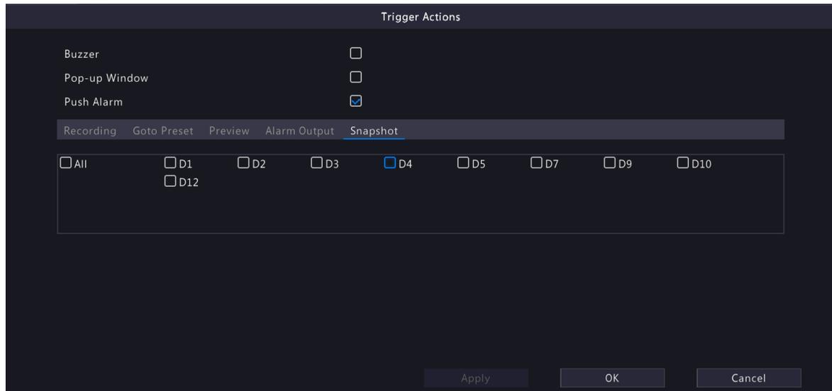
**Note:** This action is only available to certain alarm functions such as motion detection and human body detection and is not available to VCA functions.
