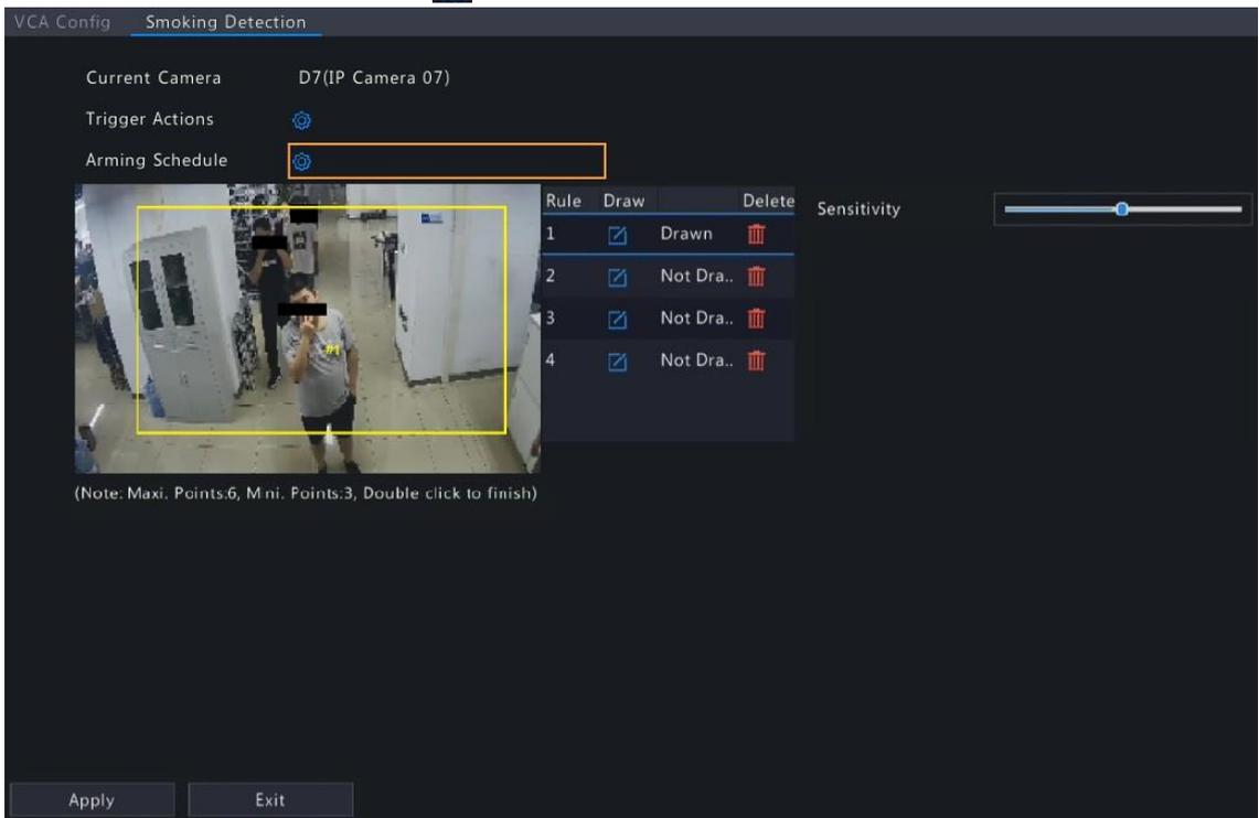
4. Set detection rules. The 4 detection rules shall be set separately. The following takes Rule 1 as an example.
