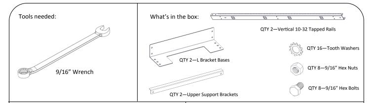
Step 1 : Assemble the L Bracket Bases to the Vertical Rails as shown below. Do this for both sides.
