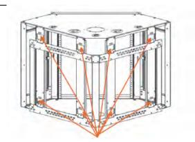
Once mounting frame is secured to corner, lift and lower the wall mount cabinet so that each of the eight (8) beveled tabs slide into the eight (8) slots in the back of the wall mount cabinet.
