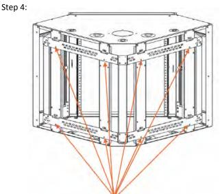
(Optional) Install wall mounting screws (not provided) for additional security in these eight (8) locations to secure the cabinet to the mounting frame.
