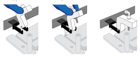
**Note:** Ensure that the back/bottom end of the Tip Arm is not resting on top of the thumb screw, causing the Tip Arm to tilt forward. Do *not* adjust the angle of the arm unless you need to calibrate the instrument.
