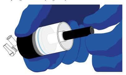
**6.** Apply a thin layer of Xiameter<sup>™</sup> PMX-200 Silicone Fluid evenly to the inside of the syringe body.
