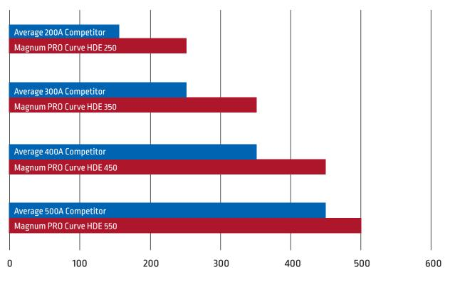
Amperage Rating at 100% Duty Cycle (Mixed Gas)
