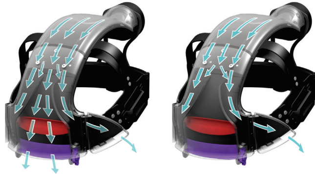
First baffle (Red) - controls ratio of air over forehead vs temples
