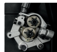
Heavy-duty aluminum two-drive-roll system
