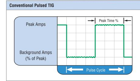
Typically from 1 to 10 PPS. Provides a heating and cooling effect on the weld puddle and can reduce distortion by lowering the average amperage. This heating and cooling effect also produces a distinct ripple pattern in the weld bead. The relationship between pulse frequency and travel speed determines the distance between the ripples. Slow pulsing can also be coordinated with filler metal addition and can increase overall control of the weld puddle.
