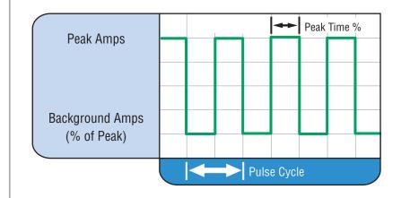
In excess of 40 PPS, Pulsed TIG becomes more audible than visible — causing increased puddle agitation for a better as-welded microstructure.
