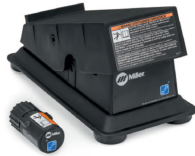
Wireless Remote Foot Control 301580 For remote current and contactor control. Receiver plugs directly into the 14-pin receptacle of Miller machine. 90-foot (27.4 m) operating range.
