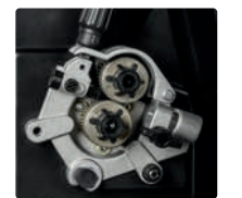
Heavy-duty aluminum two-drive-roll system
