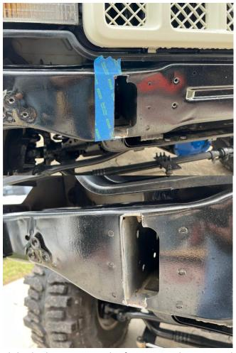
• Slide the bumper into the frame, use the existing holes on the side of the frame to locate the bumper.
