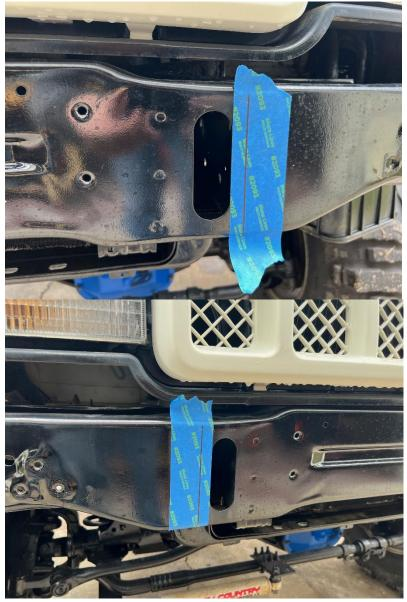
• Measure ½" over and scribe a line down the front of the frame face. The goal with this cut is to make it flush with the inside of the frame rail, it is best to be conservative with the amount cut and come back with a flap wheel and clean up what is left.
