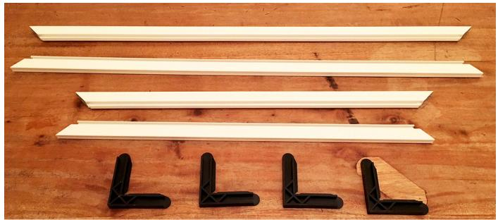
• Assemble with the corner pieces and take it to the window cavity to check how it fits before continuing. It should be able to sit within the cavity without friction, but with no more than a few millimetres clearance between each edge and the window cavity.
