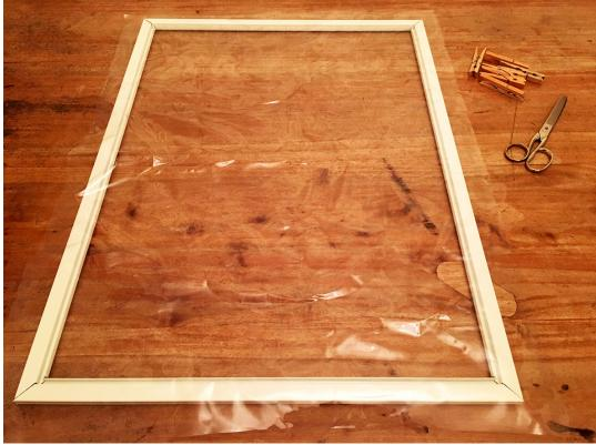
• Lay your frame down flat with the spline gutter facing upwards. Lay your vinyl on the top and flatten it out. Cut around it so that you have 50mm or so bias surrounding the frame.
