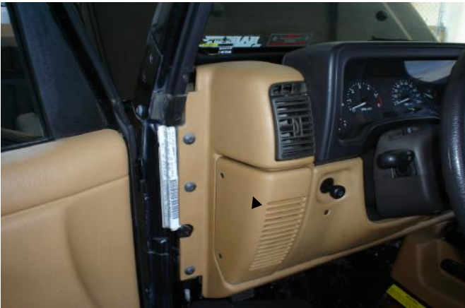
Remove Six torx bolts
