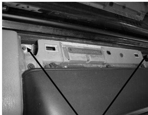
Remove all four 6mm nuts (Only one pictured)
