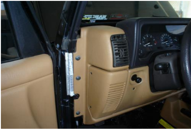
Remove Six torx bolts
