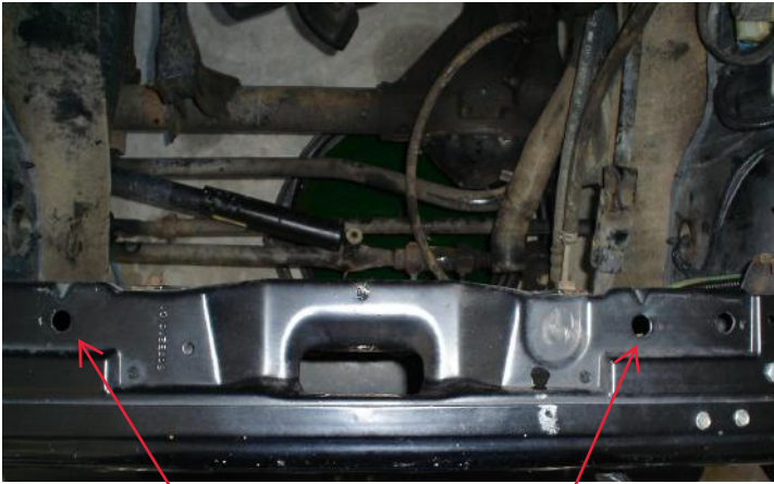
Figure 3.1 Holes for mounting Condenser
