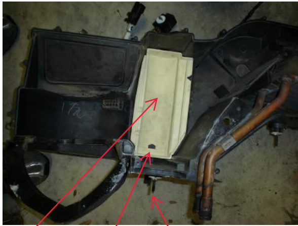
Drain reservoir Hole for drain Drain
