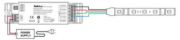
Application Circuit 4: RGBW (V+ $\rightarrow$ COM $\$  CH1 $\rightarrow$ R $\$  CH2 $\rightarrow$ G $\$  CH3 $\rightarrow$ B, CH4: W.)
