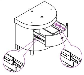
Pull the right clip upward and left clip downward at the same time, then draw the drawer box out.
