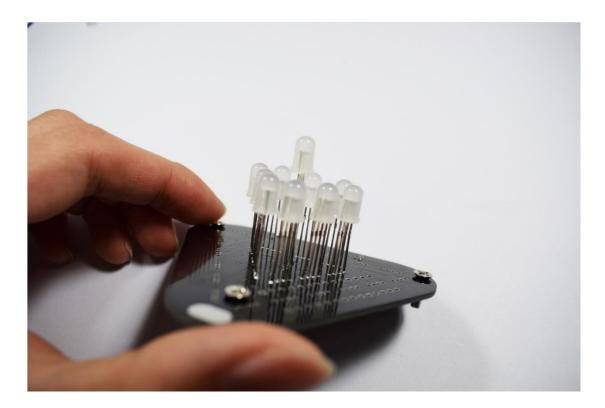
The same to the third lap.height of LED in the third circle should lower than the height of the second circle of the LED high.
