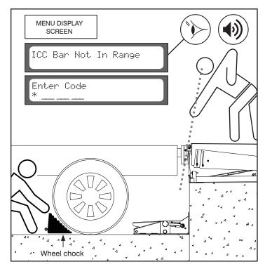
2A. Press the \* key on the keypad. The LCD screen will read 'Enter Code \*\_\_\_'.
