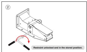
Rotate bar away from the wall to unlock. Restraint arm can descend to the stored position.
