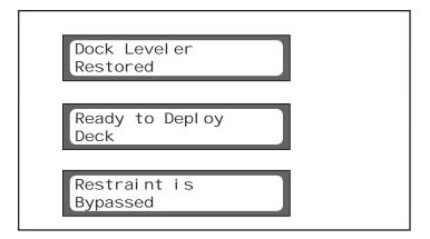
2C. Once the deck is deployed and the home sensor becomes inactive, the control panel light will turn GREEN while flashing YELLOW. This indicates that the vehicle restraint is not engaged.
