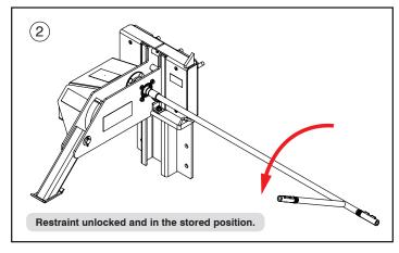
Rotate bar away from the wall to unlock. Restraint hook can descend to the stored position.
