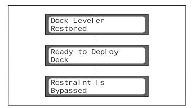
2C. Once the deck is deployed and the home/lip sensor becomes inactive, the control panel light will turn GREEN while flashing YELLOW. This indicates that the vehicle restraint is not engaged.
