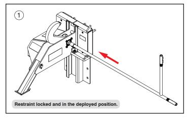
Insert unlocking bar (Part# 56-011930) into slot with pressure for leverage.
