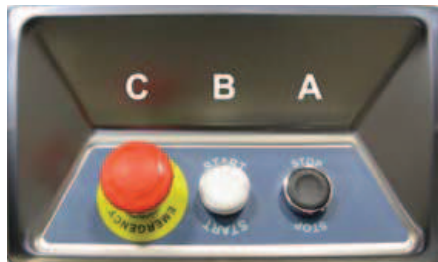
photo 1 A = STOP B = START C = EMERGENCY STOP
