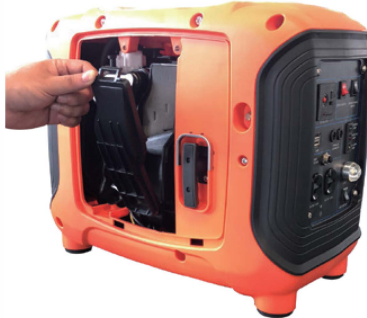
Figure 6 - Removing the air filter cover
