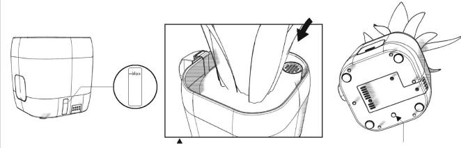
If water reservoir is dry, you may refill directly through the inlet on the top
