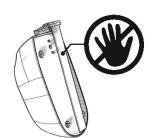
**Do not touch** the ionizer clip when the power is on.
