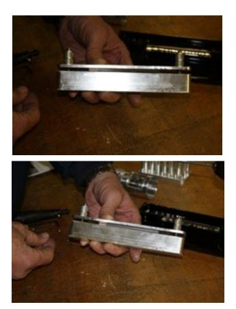
12) Place the coil holding devise with the end that the coil is on against the stop. Place the hand piece holding collar with the HP and blade in place on the coil holding devise. Run the flex shaft at full speed and with both hands and a light grip; pull the collar evenly towards you slowly. Once the cut is complete, remove the jump rings from the
