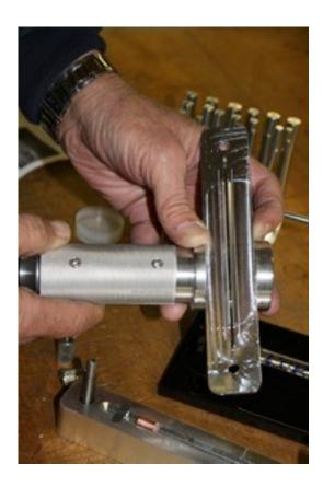
10) Snap the No. 30 HP with the holding collar on to the flex shaft. Make certain that the rotation of the blade is CCW, spinning from right to left.
