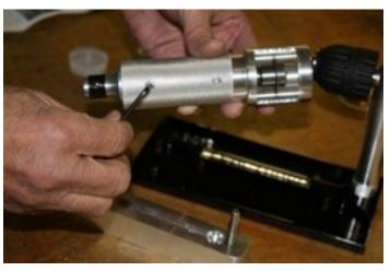
9) Place the cover over the coiled wire and replace the hold down nuts. Hold the cover down with your fingers right over the coiled wire. Tighten the nuts firmly but not excessively. Be certain that the cover is level over the coiled
