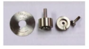
8) Slide the No. 30 Handpiece on to the handpiece Holder. Use the coil holder cover to center the blade, there is also an inscribed line that will aid you in centering the blade. Tighten the handpiece holding screws lightly, not excessively, located in the on top of the handpiece holder. The blade will now be centered on both the handpiece Holder and in the cutting groove on the Coil Holder.
