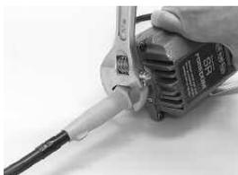
Loosen set screw on the flexible shaft motor coupling and slide shaft off the motor shaft.
