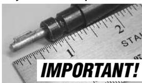
**Important Note: The shaft and sheath should be checked and adjusted (if necessary) even if you received them assembled and attached to the motor!**
