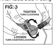
To disassemble the handpiece, use the crescent wrench or pliers to grip the graver (**FIG. 3**) and turn it counterclockwise to loosen the chuck retainer.
