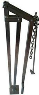
**SHEARED POST REMOVAL TOOL** (Supplied with Industrial Removal Tool) Lever open the sheared off post enough to allow the triangular head of the tool to drop down into the cavity. Hook a link of the chain to the peg at the top of the vertical lifting bar.
