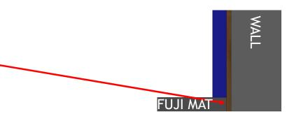
Pilot Your Holes in the Pad Lip (use a wood bit, and drill into a scrap piece) 2 Holes for each top and bottom lip will do.
