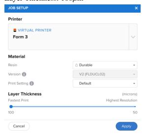
\* Please avoid any large aspect-ratio geometry (e.g. thin wall or long rod) in the object to reduce failures.
