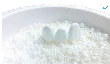
Place the restoration on the incisal edges. The pontic must rest on the sintering tray.
