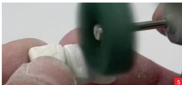
Tidy up the surface using the wheel for zirconia.
