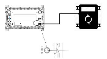
B: When multiple batteries are used in series or parallel, the external device communication line needs to be connected to the battery Link in;
