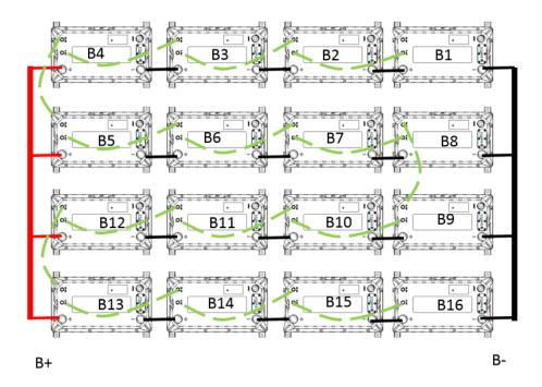
For example: 16 12.8V120Ah batteries, 4 in series & 4 in
