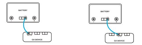
Connect one end of a CAT7 cable to the battery's CAN port and the other end to the GX device's BMS-CAN or VE.CAN port.
