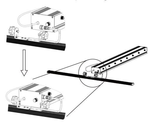
2.2 Align the lamp strips perpendicular to the driver housing, connect the female socket on the lamp strip with the male plug on the driver housing. Plug the sockets together, then twist the coupling 1/4 turn to lock. Finally, tighten the hand screw nut to hold the lamp strip in place. Repeat with each LED lamp strip.
