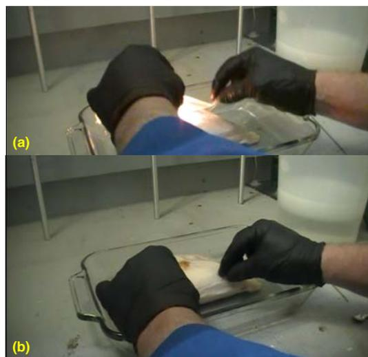
**Figure 3:** ClearCool hydrogel was applied directly over the top of burning WP. The white hot glow of the WP can be seen in (a) as the ClearCool is situated over the WP. As soon as the ClearCool is lowered over the WP (b), the flame is instantly and completely extinguished. The reddish dot in (b) is from charred chicken skin on the contact side of the ClearCool.
