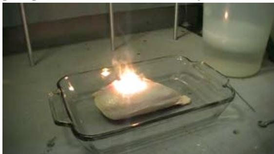
**Figure 2:** Ignition of white phosphorus. The apparent diameter of the burn is overstated from the camera exposure to burning MeOH around the WP. The area around the white hot WP was actually about 2 cm in diameter. Once ignited, the WP burned as intensely as expected. The large beaker in the background was to be used as a safety quench in case the WP tube caught fire. As it turned out, the beaker of water was not needed and the MeOH-coated WP was quite easy to work with safely in the hood.
