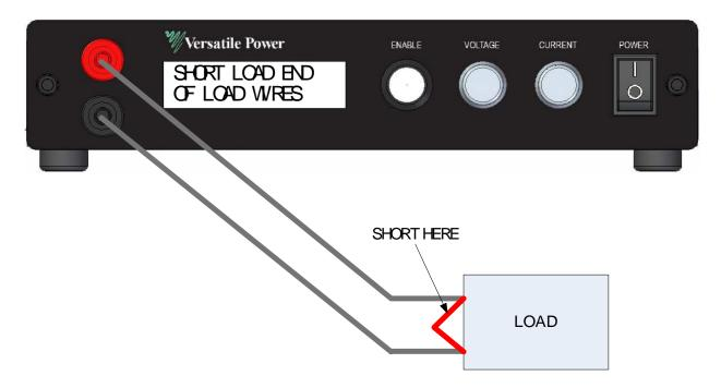
It is important that a good short with heavy wire is made as failure to do this will result in a poor remote sense calibration.
