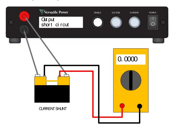
When the power supply is configured as in the figure above, press the Enable button. The following screen will now appear:
