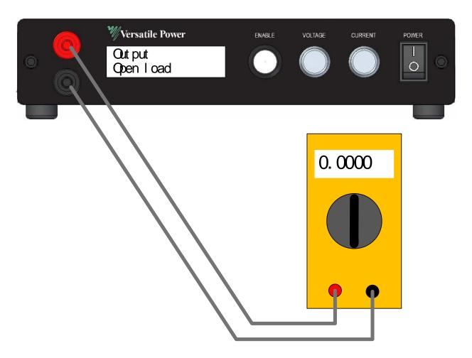
When the volt meter is connected, press the Enable button. The following screen is an example of what will appear.
