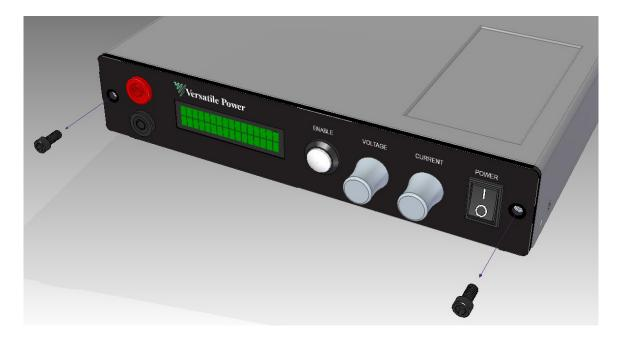
4) Hold the rack mount plate in front of the power supply front panel and secure with the new screws provided with the rack mount plate. Do not use the original screws as they will be too short. See figure below:
