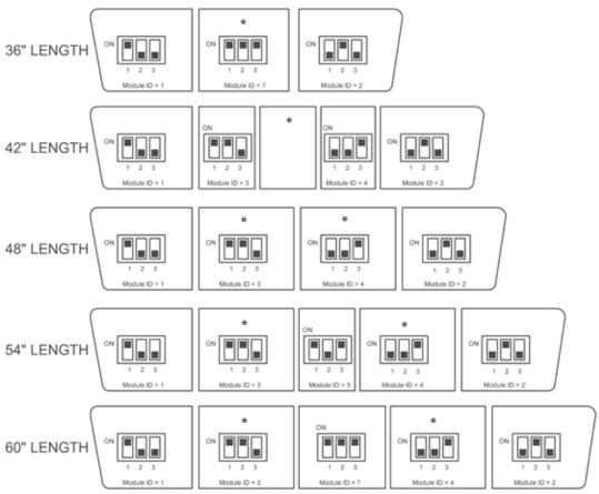
\*Controller Board Location, location will match wire side exit (Refer to Page 6 for DIP Switch Settings)
