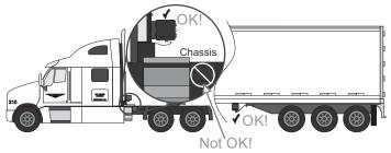
Step 2: Dump the air from the suspension system.
