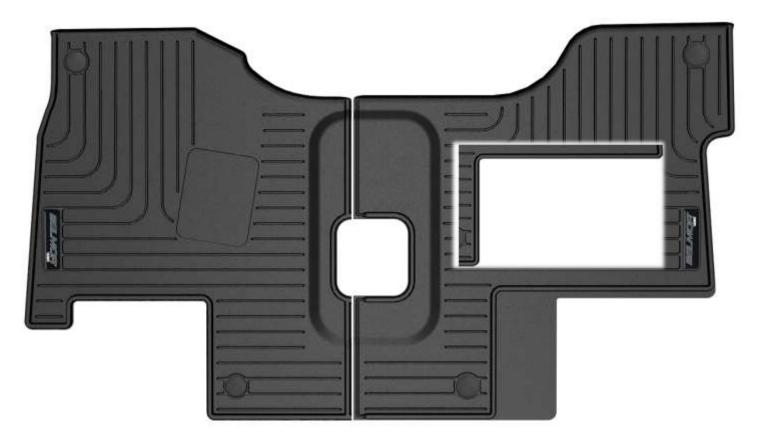
The trim for the front passenger side liners are highlighted above. These trim accommodate seat variations available in truck models. When trimming, leave the protective rib wall (see images of trim in insert view).
