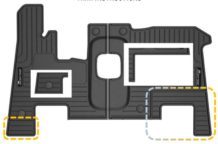
Trims for the front driver and passenger side liners are highlighted above. These trims accommodate fire extinguisher positions on the **driver's side and seat base variations on Peterbilt** models. When trimming, leave the protective rib wall on the liner (see images of trim in insert images).
